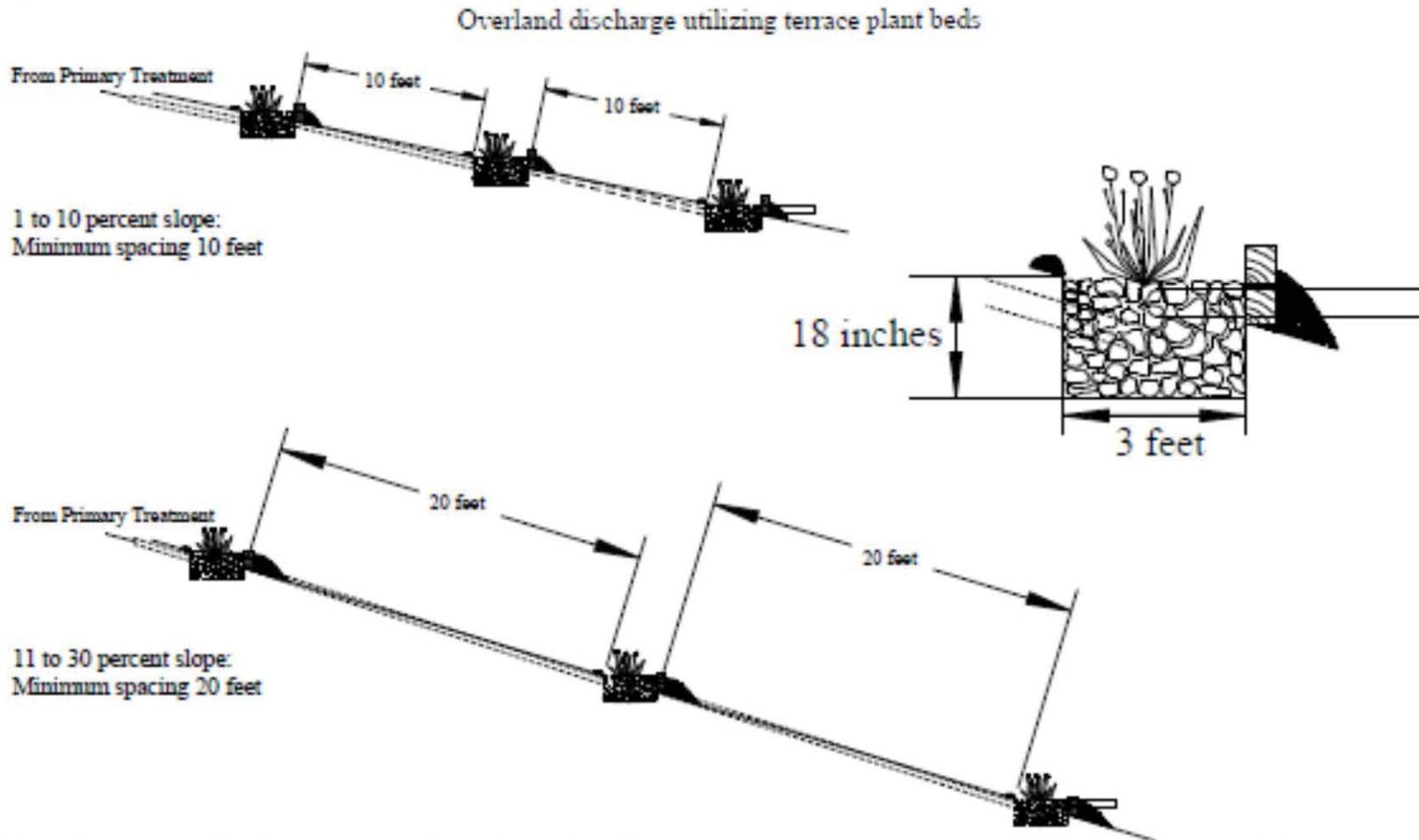
Further absorption of the effluent could be enhanced with the addition of plantings (canna, calla lilies, elephant ears, etc.) in a bed following the distribution manifold.
