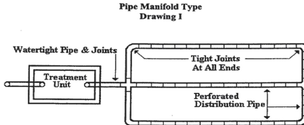
In absorption bed systems where the entire infiltrative surface is at one elevation closed loop networks may be used. The distribution pipe is laid level over the media filled excavation and the ends connected together with additional pipe with ell or tee fittings.
