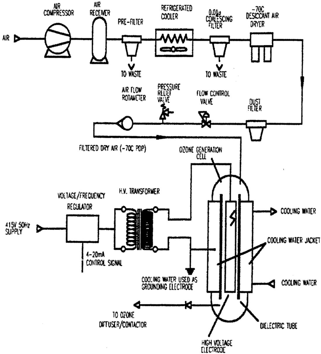
Fig. 1 – Typical Vertical Tube Ozonator Process Flow Schematic
