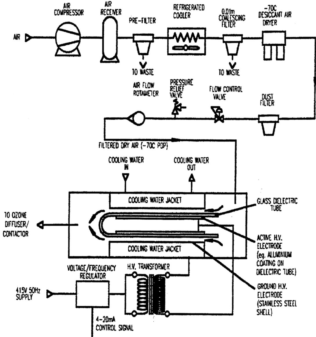
Fig. 2 – Typical Horizontal Tube Ozonator Process Flow Schematic
