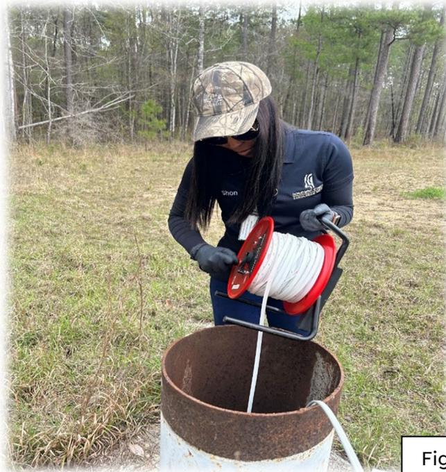
Figure 19. Shonquatta Williams (MSDH) collecting a water level reading from a well at the STS Site.
